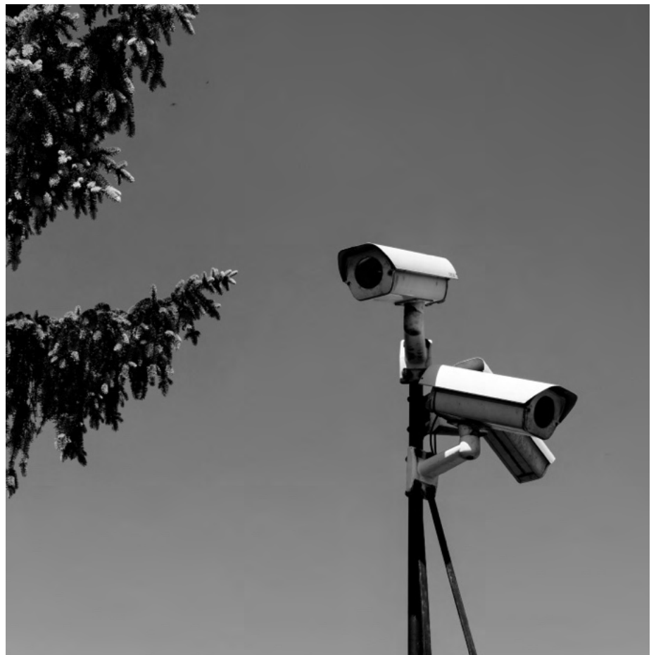
Fig. 15: Extruded Bullet Cameras (Jakubowski, 2020)
