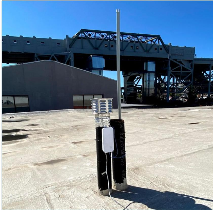
[FIGURE 20 ▲ ] A LoRaWAN gateway and antenna installed by NYU on a roof in Gowanus, Brooklyn. Photo: NYU CUSP
