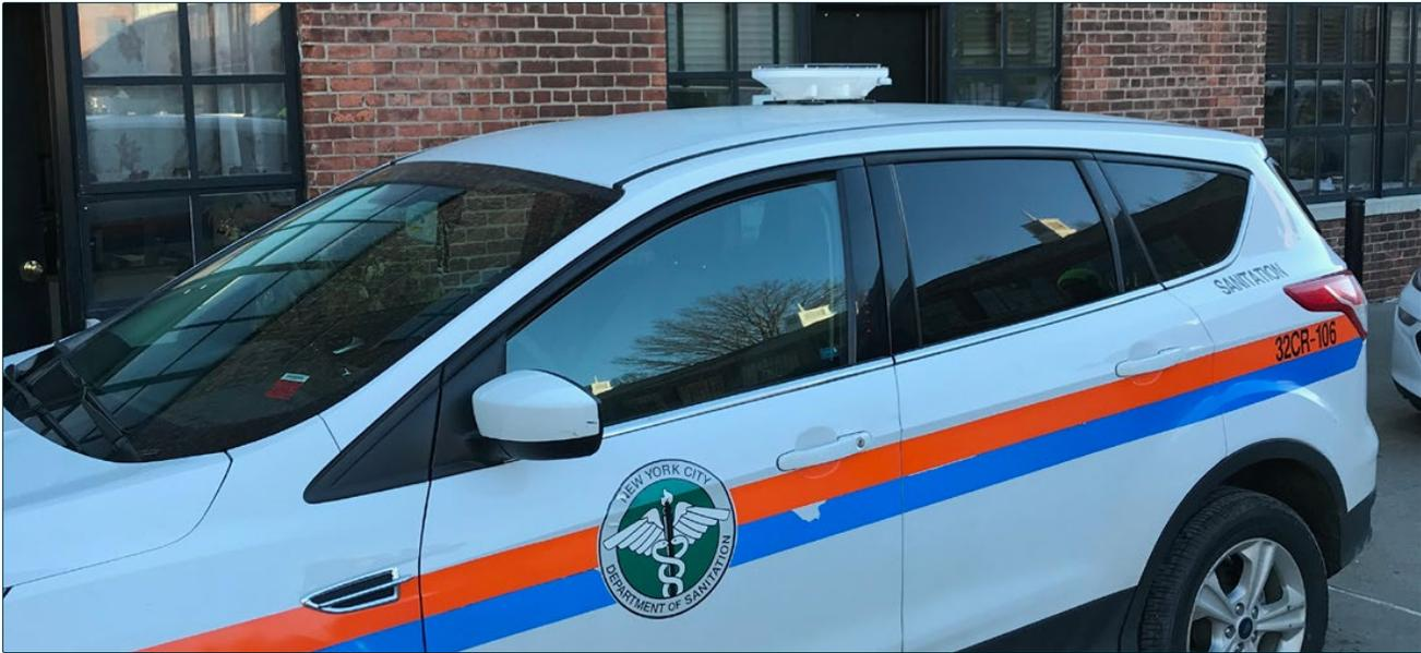
[FIGURE 15 ▲ ] An MIT CityScanner sensor node on top of a New York City Department of Sanitation vehicle.
