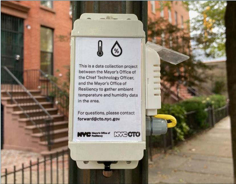
[FIGURE 16 ▲ ] A temperature sensor installed in Brooklyn for a rapid IoT pilot with MOR.
